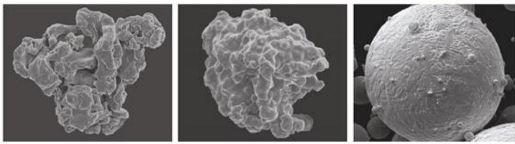
Figure 4: Examples of powders with different morphologies. [8]
