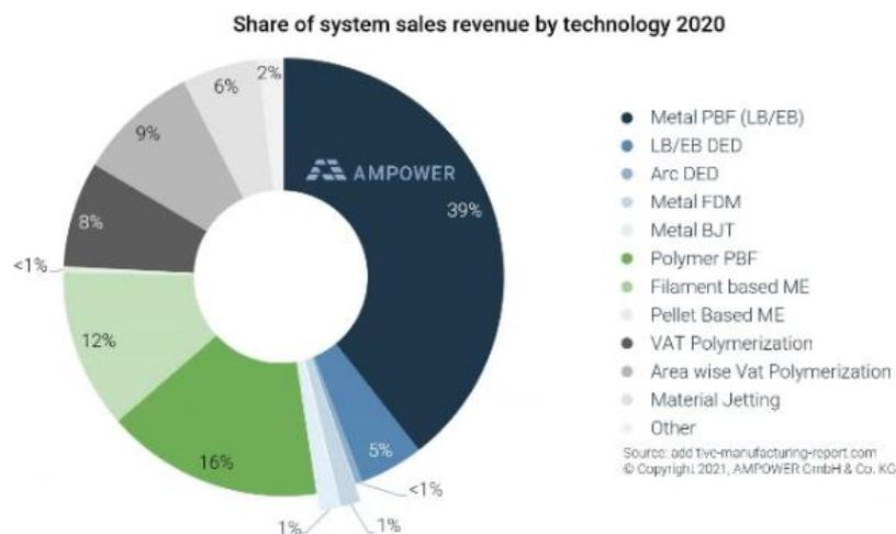
Figure 1 - Overview of System Sales in AM for the Year 2020 (copyright: AMPower 2021)
